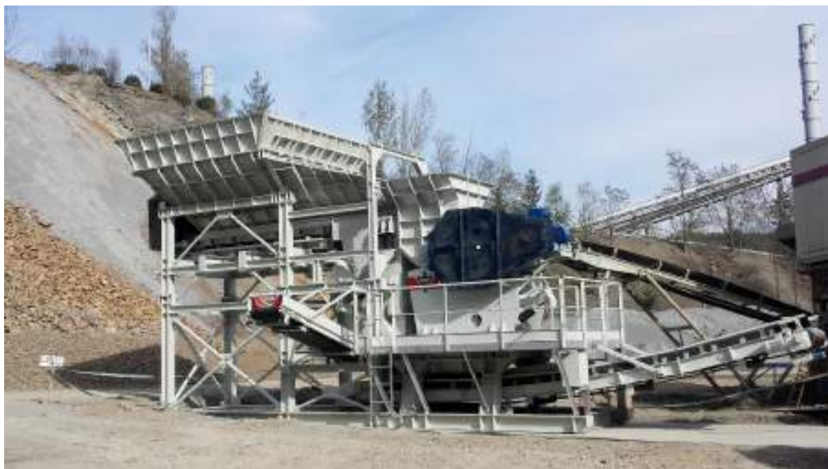
KÁMEN ZBRASLAV (Czech Republic) – Portable crushing unit with jaw crusher DC 105 x 80 S
