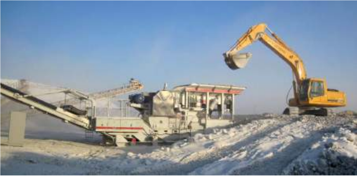
KRASNOTURYINSK (Russia) – Portable limestone processing plant 120 tph - SCU 95x70, SCU 9, VTK 160x500/3
